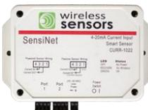
The CURR-1022 data acquisition Smart Sensor is a wireless current sensing device which accepts two 0/4-20 mA signals. The CURR-1022 has on board batteries for complete tether free operation or can be equipped with an external DC (10-30VDC) power supply which will simultaneously power two loop powered transmitters and the CURR-1022.
