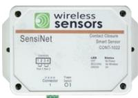
The CONT-1022 data acquisition Smart Sensor is a contact monitoring device which accepts two contact inputs and is a member of the SensiNet wireless sensor network. It continuously monitors the state of its inputs and reports their status on a selectable reporting interval and will also report any change in status immediately for real-time alarming. The CONT-1022 can be used with a variety of switches including mechanical, IR, and magnetic .
