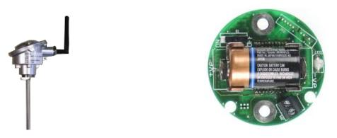
The model SB-PT100 will accept any PT 100 RTD as its sensor input allowing customers to choose best in class components for their measurement systems or Wireless Sensors can provide sensor, housing and transmitter as a complete package for single source simplicity.
