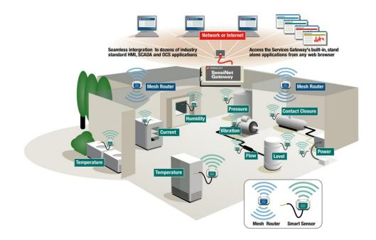
Figure 1: Architecture of a SensiNet wireless sensor network.
